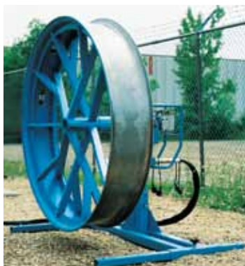
50" (1,270 mm) diameter capstan on Remote Mounting Stand.
